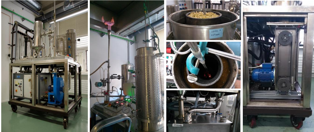
Open-top gasification system
